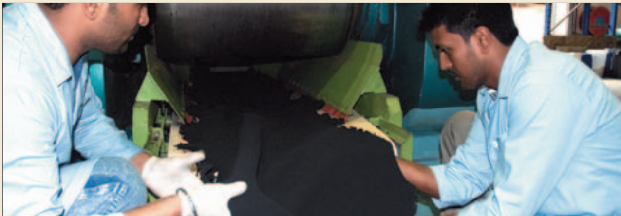
Operators at Green Rubber's plant feed de-vulcanized tires into a crushing machine that will reduce the material to rubber that can be used in a range of industries
